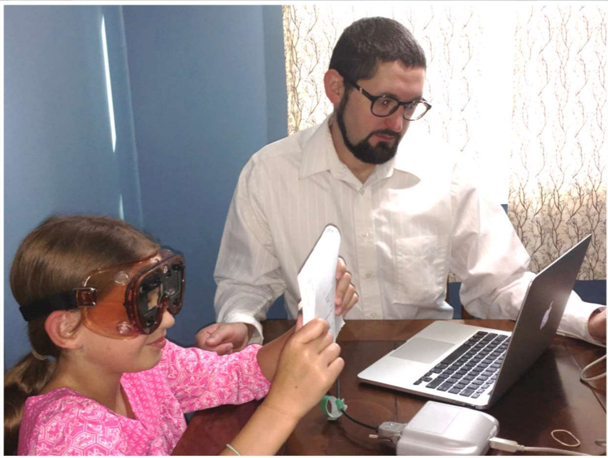
Figure 1. Student reading text from a normed test booklet while eye movements were recorded using the Visagraph.
