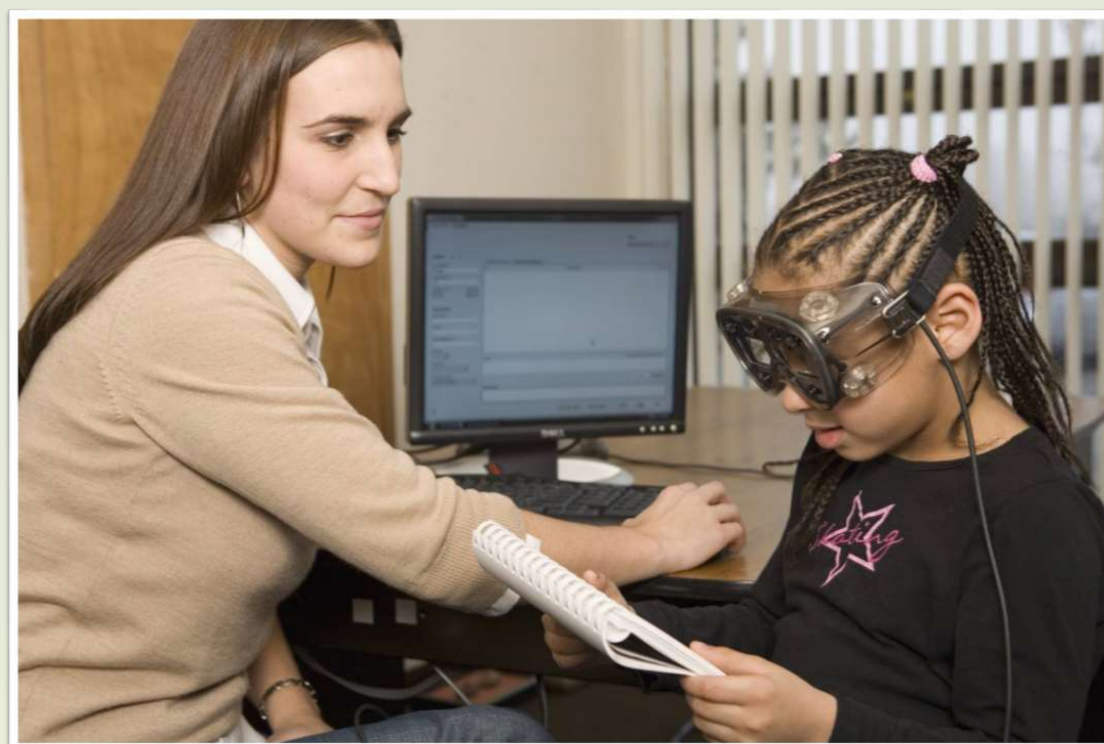
Figure 1. Student reading text from a normed test booklet while eye movements were recorded using the Visagraph.
